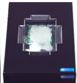
Scanner without Cryoprotection™
