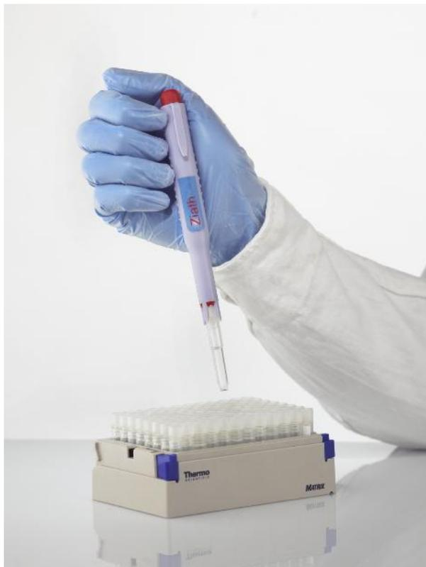
The Tube Picker simplifies retrieval of tubes, minimises heat transfer and reduces the risk of cross contamination.
