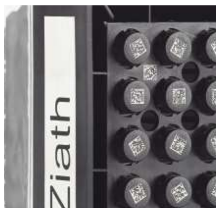
2D barcode on the underside of the rack matches the linear barcode etched on the side.
